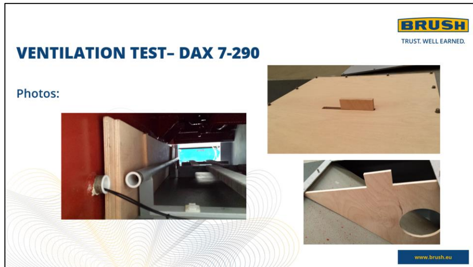
Image 9 – Transfer ducts blocking by using woody covers with appropriate cross section holes
