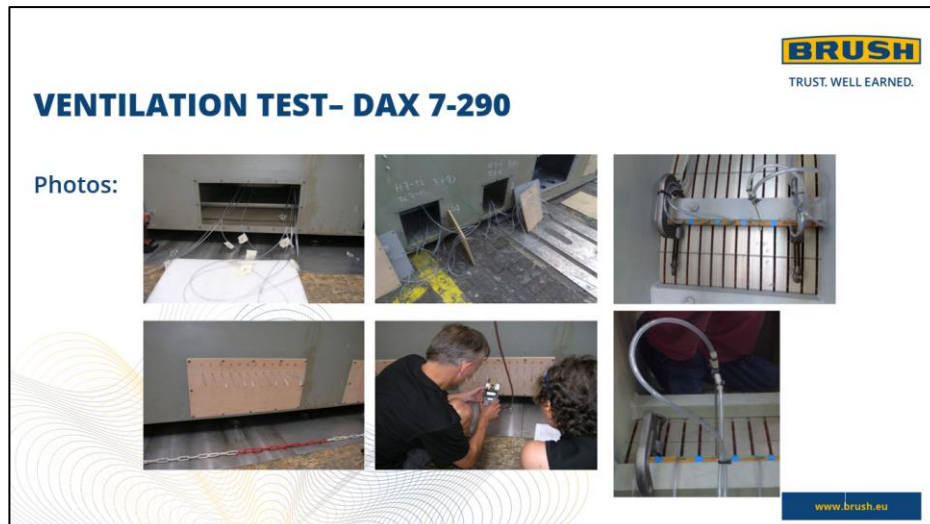
Image 7 – Stator ventilation measurement
