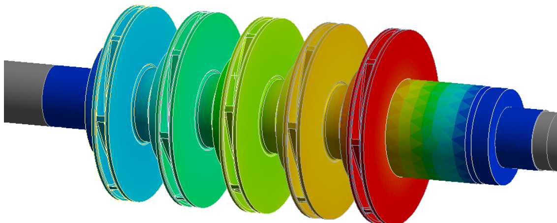
Image 14 – Pressure import - rotor (structural analysis, Optimal Q, Grooved stator)
