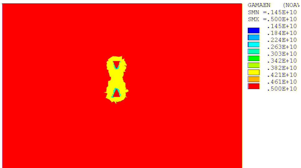
Figure 7. The distribution of electric conductivity \gamma , t=0.4\mu s
