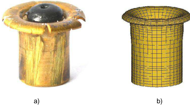
Image 12 – Comparison of the character of deformed bullet: experimental (a) and simulation (b)
