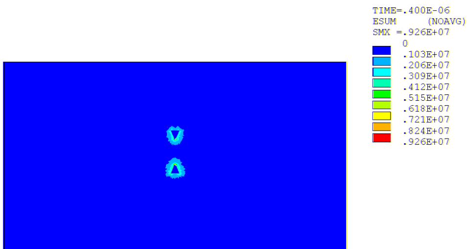
Figure 10. The module distribution of electric intensity E , t = 0.4 \mu s
