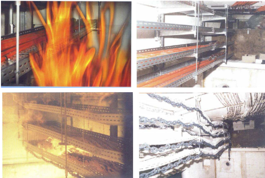
Figure 2 Experimental test of the cable way structures in TU laboratory Braunschweig [13]
